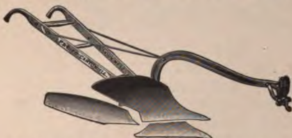
FIG. 76. Plow with interchangeable moldboard and share.
